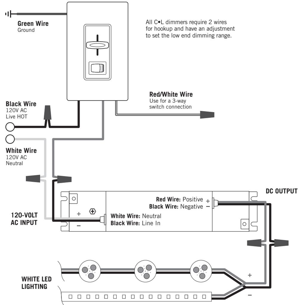
Power supply is for direct wire only. Includes NEMA 1 listed metal enclosure. After removing knockouts, install suitable strain relief cable clamps and route wires appropriately to fit installation location.
